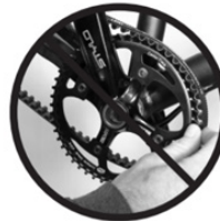
Mounting the tensioned belt with a lever, and/or by rotating the cranks
