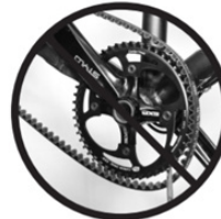
Mounting the tensioned belt with a lever, and/or by rotating the cranks
