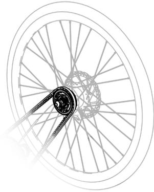
**Step 2.** Carefully insert the wheel axel into the dropout and align the brake rotor inside of the brake. If necessary, loosen the MOD-Nut to make this step easier.
